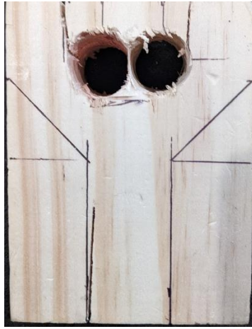
Figure 17: Top View of Errors in Drilling
