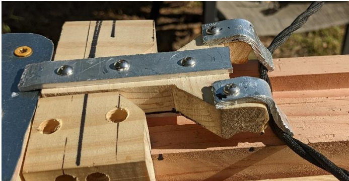
Figure 24: Repaired Claw with Aluminum Fingers
